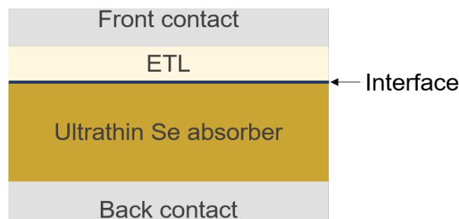
Figure 1: Simplified Se solar cell structure used for SCAPS simulation.
